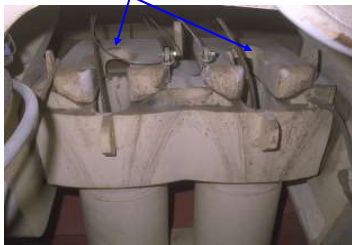
Base of turret double Chain stopper/ trumpet assembly
