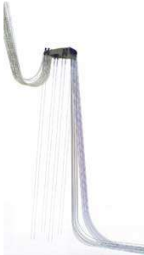
Buoyancy Supported Riser (BSR) Subsea 7 - Guara-Lula NE field, Brazil (Ref: OTC2014 - 25165)
